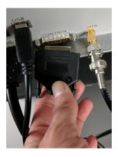
Interlocks are common safety features of industrial lasers. The DB15 connector simply shorts out two of the pins, which then connects two halves of a circuits, which in turns allows the laser to turn on. Before continuing, please watch the VIDEO called HOW TO OPERATE THE FIANIUM LASER on our website. Then turn on the laser power supply by pushing the red toggle switch at the back of the power supply. You have to wait for about ten minutes to allow the laser to warm up (it has a built-in timer).
