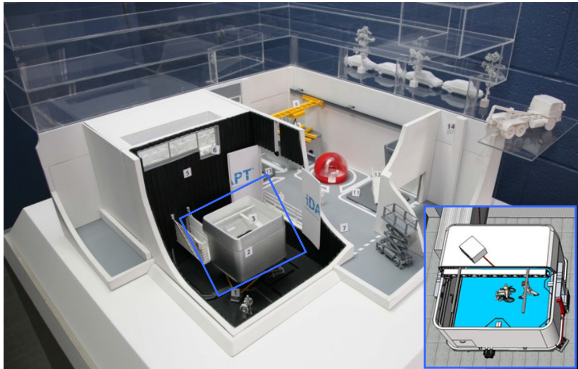
Figure 4: A model of the iDAPT Challenging Environments Assessment Laboratory (CEAL) showing the winter simulation environment (inset) mounted on the motion simulator platform. Other laboratory payloads can be seen in the background together with the overhead crane.
